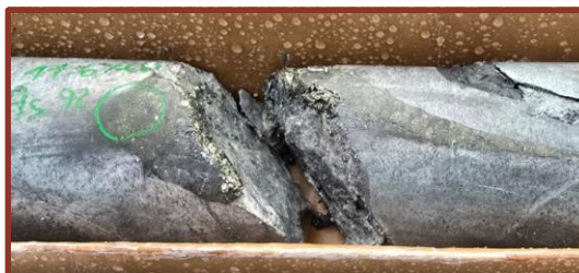
Chalcopyrite sulphide within a c-type vein within altered porphyry from 400m in 25LLDD0070
