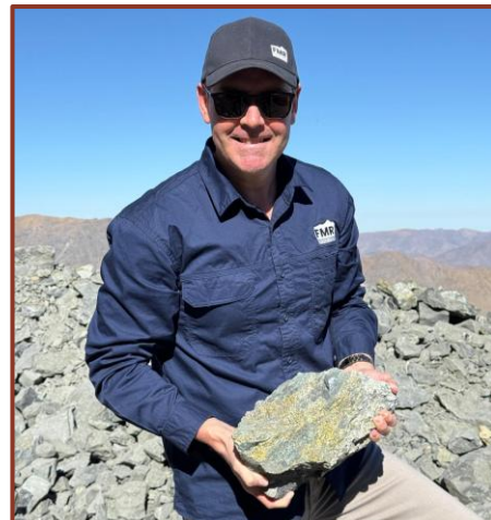
UNDERGROUND MINERALISATION: FMR Managing Director Oliver Kiddie, holding an underground sample from the La Martuca prospect, showing copper sulphide hosted in structurally controlled quartz-sulphide veining.
