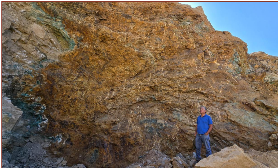
Artisanal mine exposure of large-scale copper-iron mineralised breccia and carbonate replacement style mineralisation
