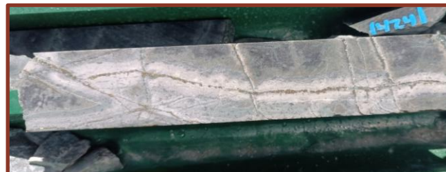
Pyrite-Chalcopyrite sulphide veining with albite selvages from 1,434m downhole in 25LHDD071
