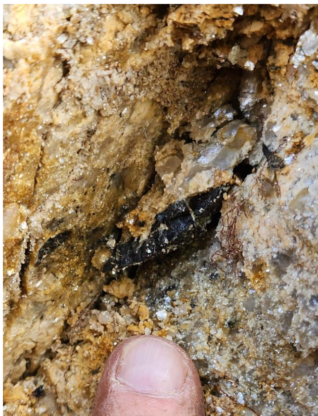
Figure 4: Sample WWP001 (1.09% Sn) - cassiterite in a greisenous pegmatite boulder from the floor of the historic Walwa open pit
