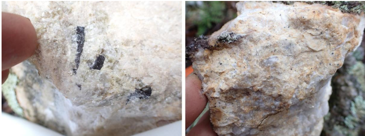
Figure 5: Sample WWP003 (0.61% Sn) - cassiterite in coarse aplite-pegmatite from outside the northern pit wall (left) and sample WAS001 (0.40% Sn) from the Mt Alwa South dyke (right)
