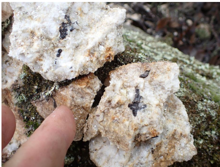
Figure 4: Sample WWP001 (1.09% Sn) - cassiterite in a greisenous pegmatite boulder from the floor of the historic Walwa open pit
