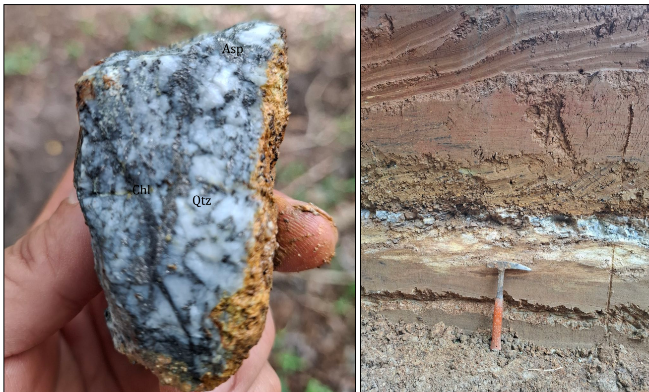
Figure 7 (left): Photograph of sample 114054 from 26TRCM005 which assayed 1.9 g/t gold and was collected from a 3-7 cm quartz vein (Qtz 60% visual estimate) with massive arsenopyrite (Asp 30% visual estimate) and chlorite (Chl 10% visual estimate) fracture fill.
