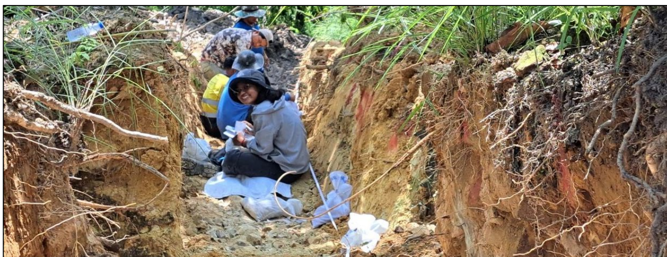
Figure 1: Unity geologists sampling trench 26TRNC001 at the Ngot Central Prospect. Trenches were shallow extending into the highly weathered saprolite, just below the soil profile.
