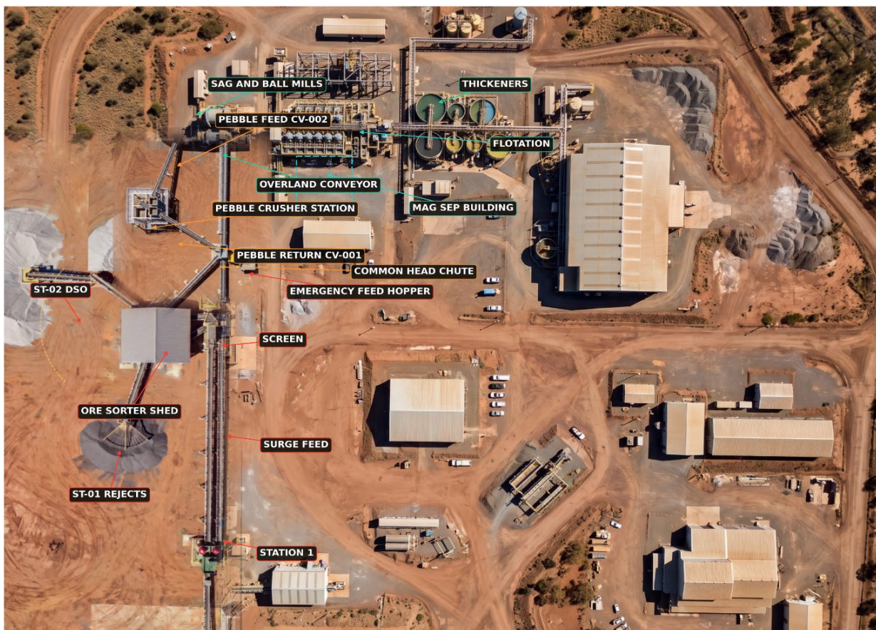
Figure 17 Nova plant, new front end on the as-built aerial (conceptual)
