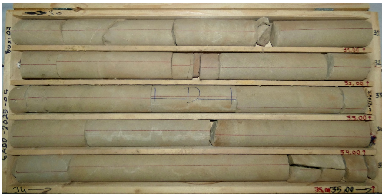
Figure 1 – Diamond drill-core from hole GADD-05 – 30m depth to 35m
