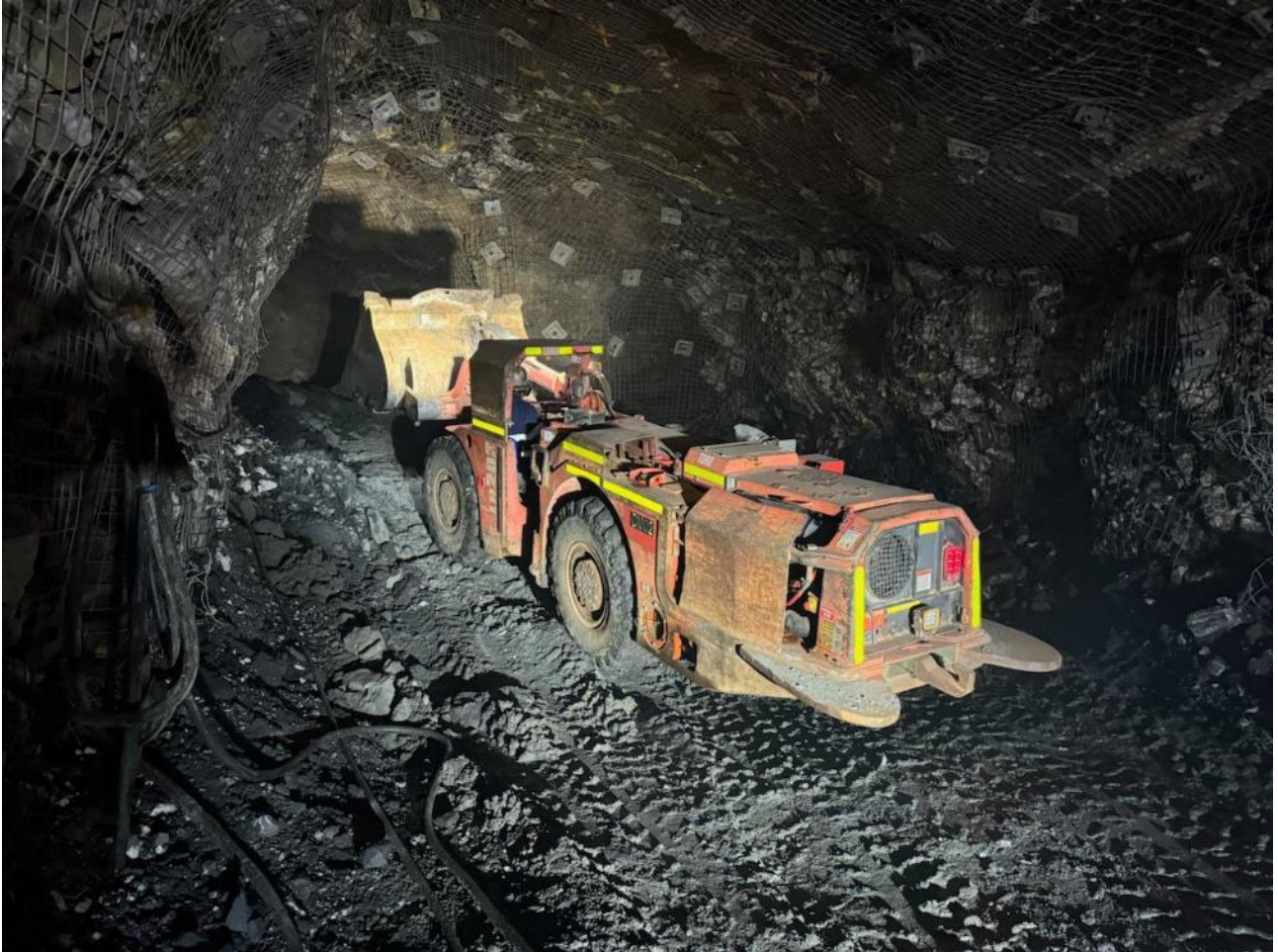
Figure 5: Cream Mining loader cleaning development headings at Paulsens underground
