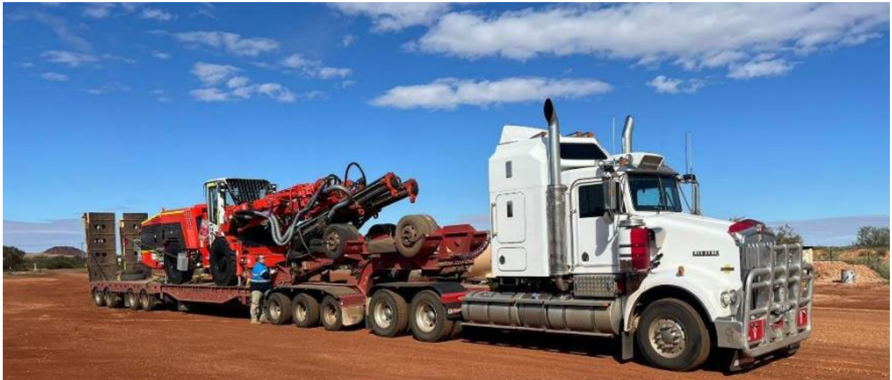
Figure 3: Unloading of DD421 twin boom jumbo as activities at Paulsens ramp up
