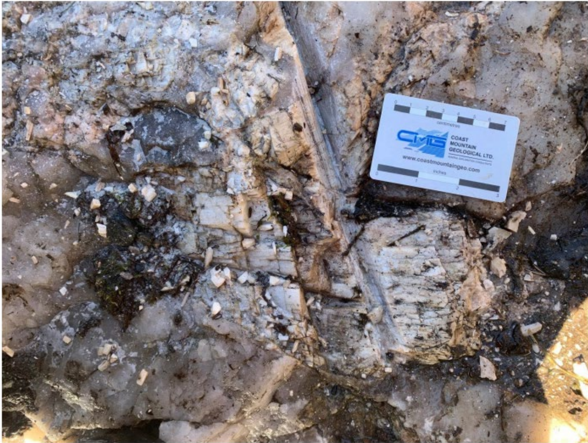
Figure 4 – Coarse spodumene at Pegmatite 7 (assays confirm grades up to 5.12% \text{Li}_2\text{O} ).
