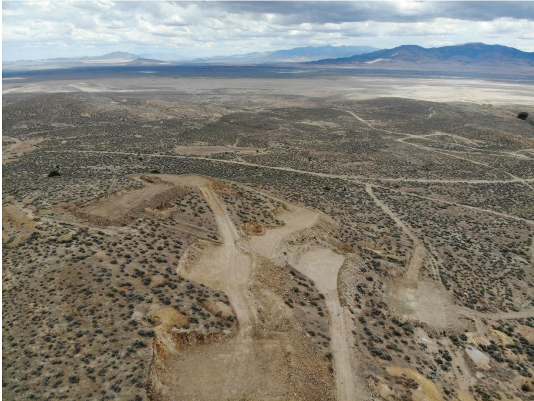
Figure 2: Aerial view of the Keystone Mine, with pads prepared for upcoming drilling campaign. Historic Keystone Mine workings can be seen in the lower left, along the north striking main Keystone Vein.
