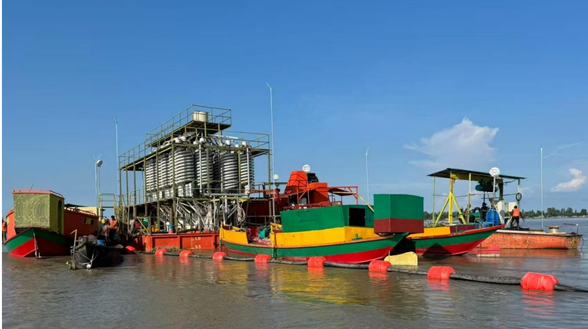
Image: Everlast's larger spiral platform at the Gaibandha project
