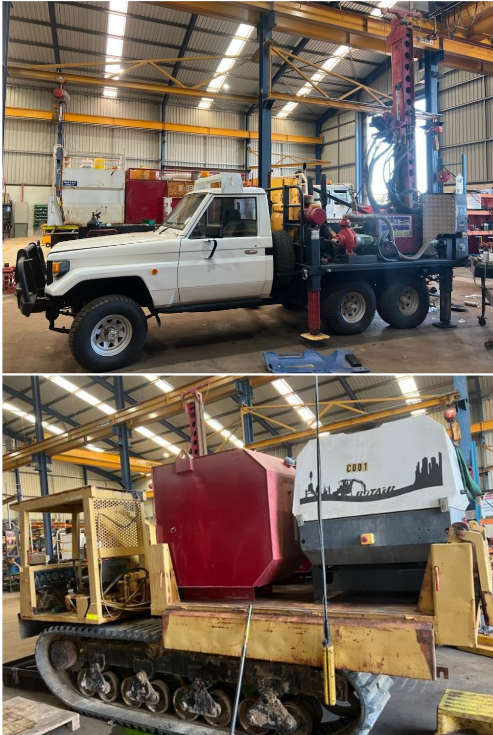
Figure 1 – Toyota Mounted drill rig and Marooka support Rig
