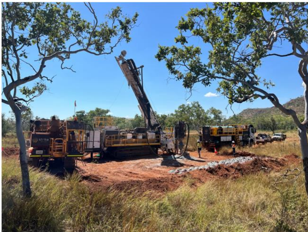
Figure 2: RC drilling during the 2026 program at the Speedwah Fluorite Project
