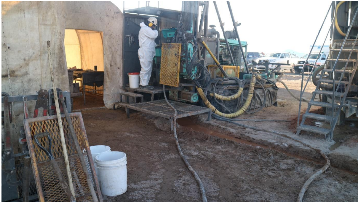
Figure 2. Drillers commencing first 30m with HQ diamond drill on well TAM 24-03.
