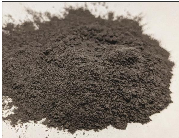
Figure 3: Antimony sulphide (37% Sb) precipitated from leach liquor 6
