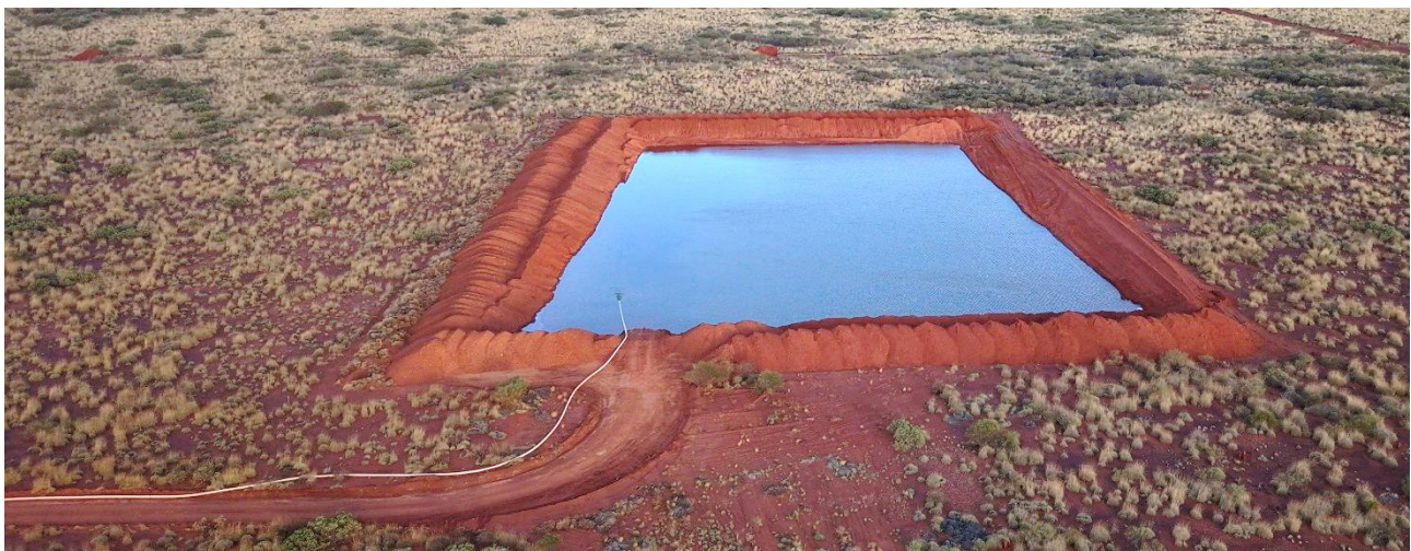
Figure 8: Water sump for long-term pump testing
