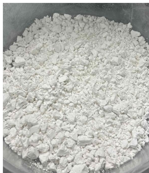
Figure 6: Hydrated niobium oxide precipitate (before calcination)
