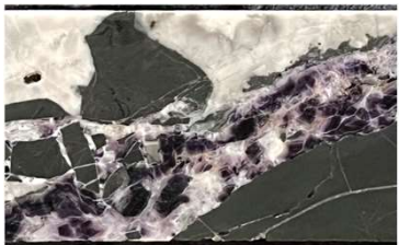
Quartz-chalcedony-fluorite breccia fill at 143.7 m in 309DD22011. In an interval of 5 m @ 9.73 g/t Au from 143 m. (HQ Core)
