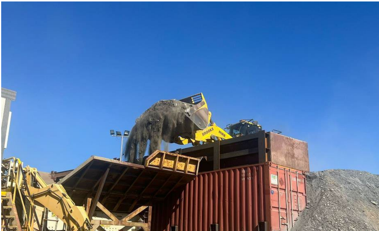
Figure 1: Crushing underway – low-grade commissioning Ore being tipped into crushing circuit as wet commissioning commences.
