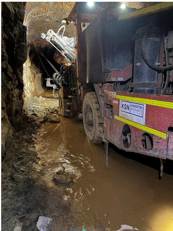
Figure 2: Kingston's first jumbo and underground loader in operation. The focus has been on re-entering and cleaning out previously flooded workings and to re-install ground support.
