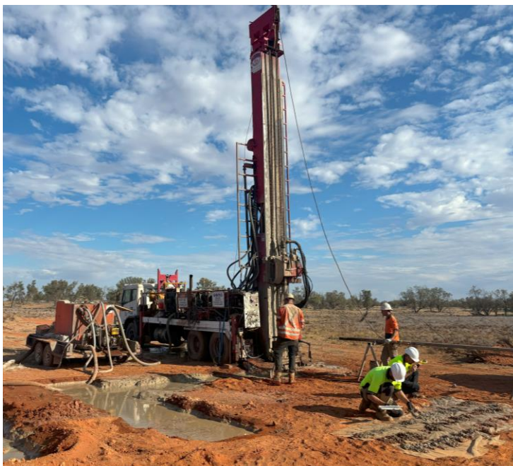
Photo 1. Drilling rig in action, targeting extensions of the Oban Uranium Deposit.
