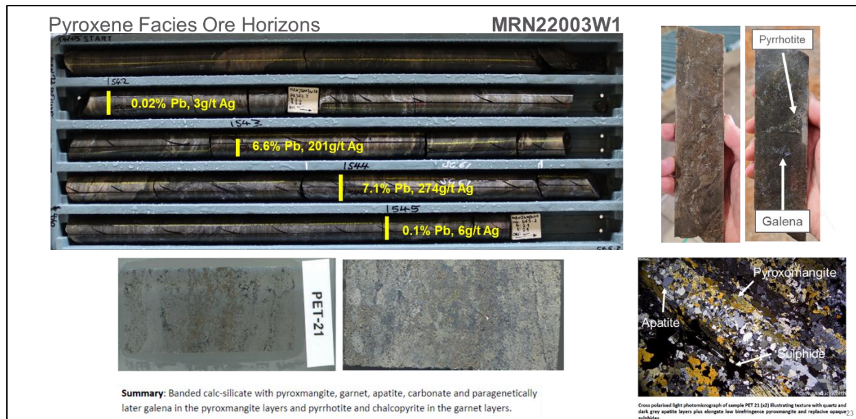
Figure 9: Pyroxene facies silver-lead mineralisation
