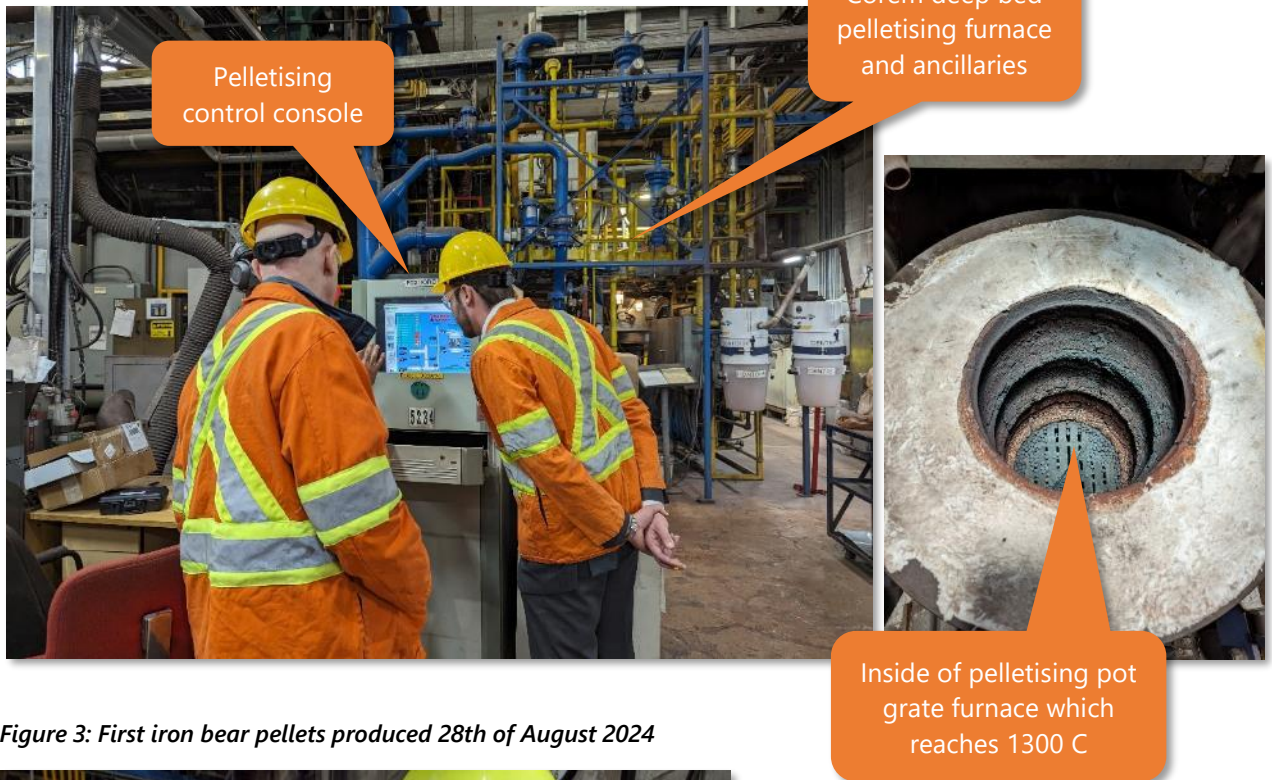
Figure 2: Corem pelletising pot grate furnace and control console
