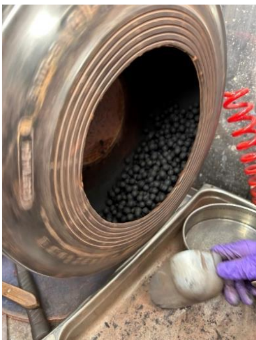
Figure 1: Photo of green balls being produced from iron bear concentrate
