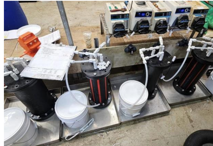
ISCR vessel setup (top), core sample (lower left) and vessel packing (lower right)
