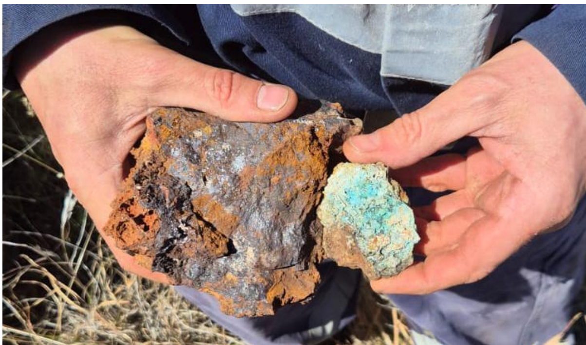
Figure 3 - Gossan outcrop (482389E, 7438704N) showing classic ex-sulphide boxwork texture identified at VT1 immediately along strike from outcropping Oonagalabi Formation marble with oxidised copper mineralisation present.
