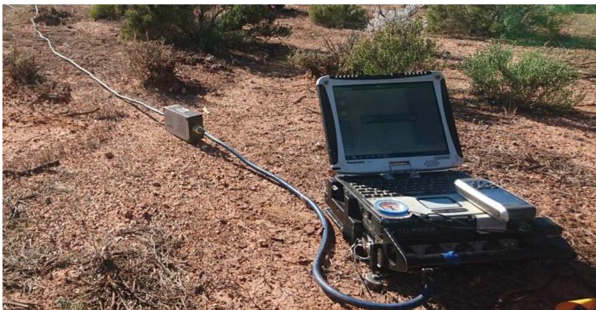
Picture 1: In Field EM survey station.
