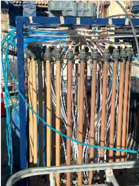
Figure 13-10: Cobalt Loading onto BPA resin.
