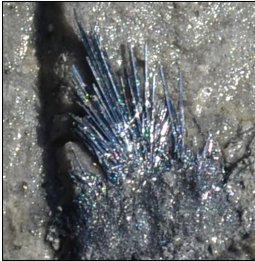
Figure 1: Stibnite (antimony sulphide) needles in fracture in core from BPD08. Antimony containing minerals at Bulla Park are tetrahedrite and stibnite
