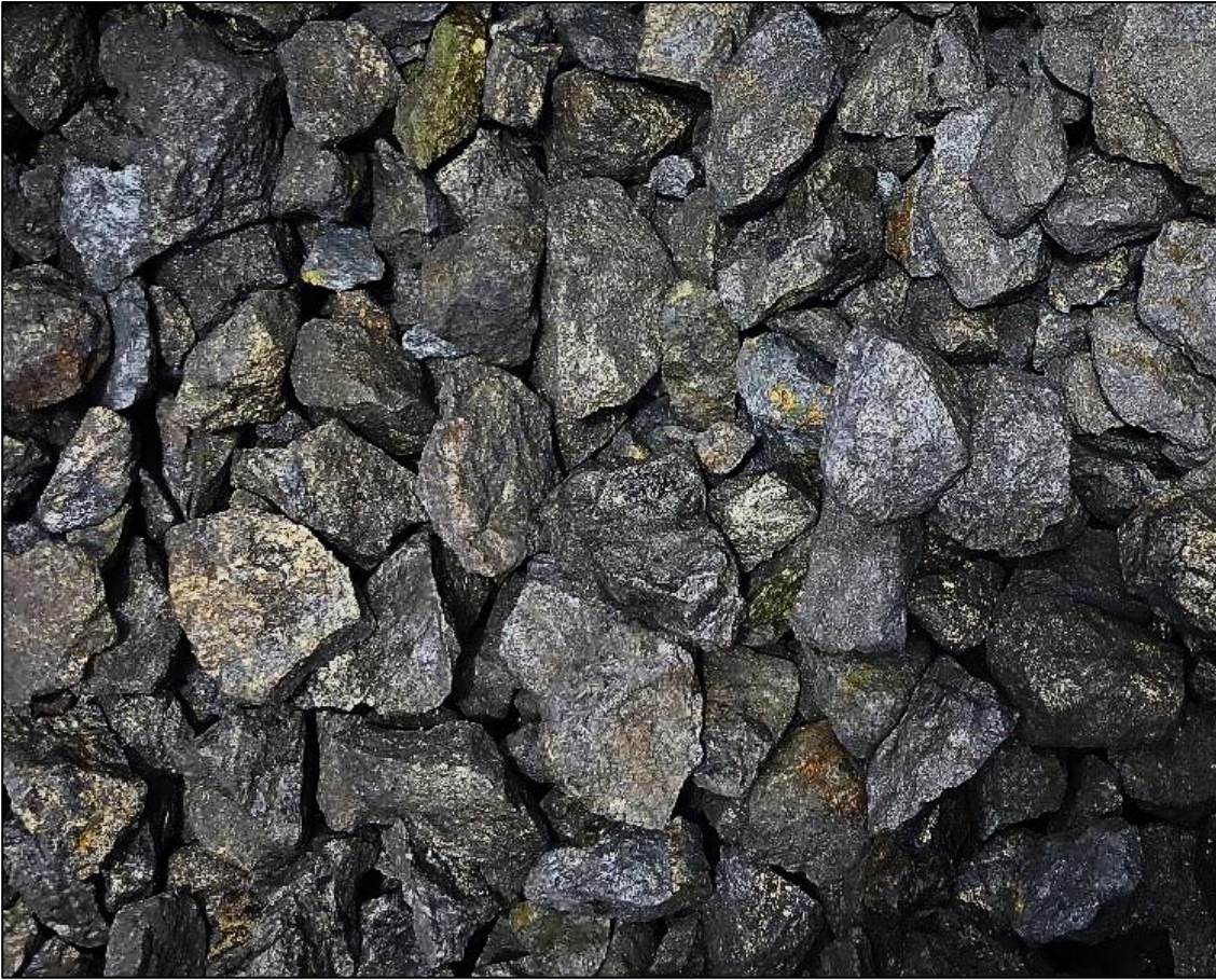
Photo 5. Mined and coarsely crushed Montezuma mineralisation. Representative sample assays of mineralisation only batches averaged 9.02% antimony (Sb), 769 g/t silver (Ag) and 15.47% lead (Pb)
