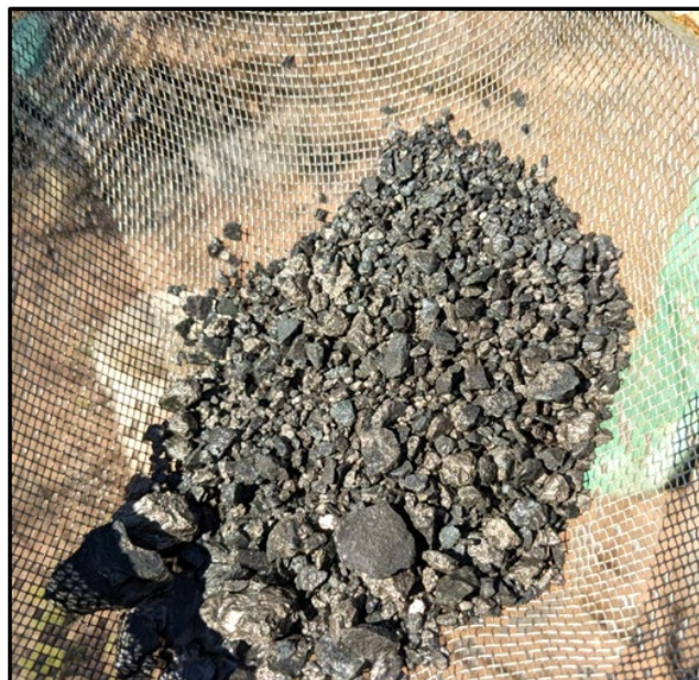
Figure 13 – Disseminated and matrix sulphides in RC drill chips from Jimberlana South (53m in NRC455)
