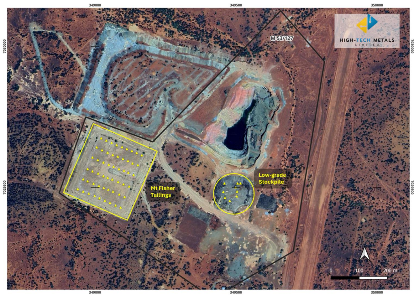
Figure 1 - Mt Fisher (M53/127), September 2025 drill collars (yellow triangles). Collar details in Table 1 below.
