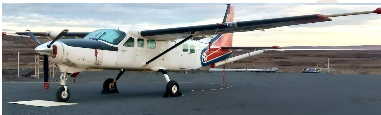
Figure 1: Sander Geophysics' Cessna Grand Caravan is flying a ~1,500km 2 Fixed-Wing Magnetic Gradient Survey at Coppermine using 3 cesium vapour magnetometers (two wingtip and one tail stinger-mounted). Now ~20% complete, the survey aims to identify demagnetised zones linked to potential mineralisation.
