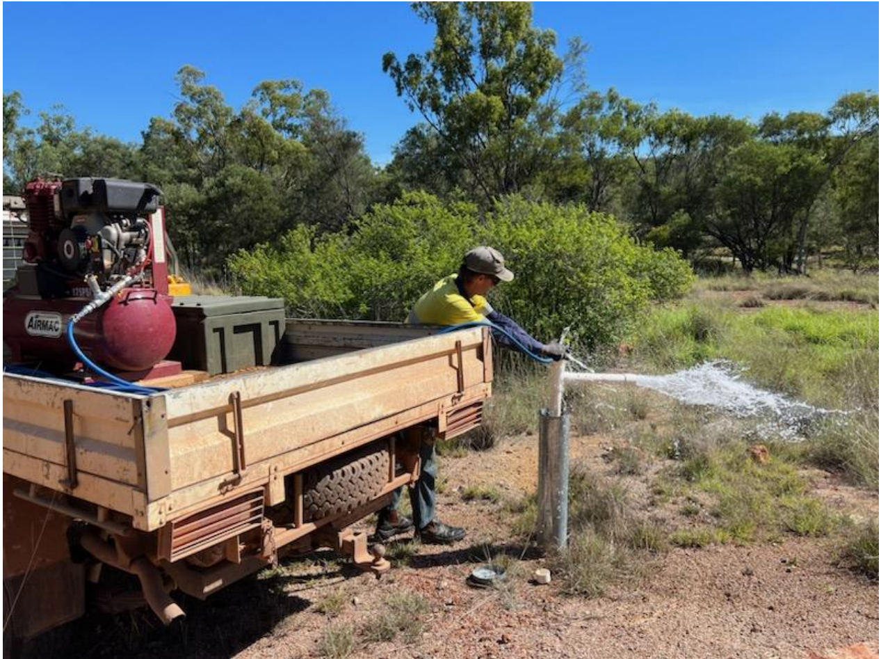
Figure 37: Groundwater sampling at Yandan
