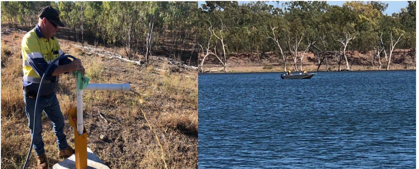
Figure 2: Yandan Gold Project - Ground water bore monitoring and water sampling at various depths in the open cut mine completed during the year, as part of the environmental water quality management requirements.
