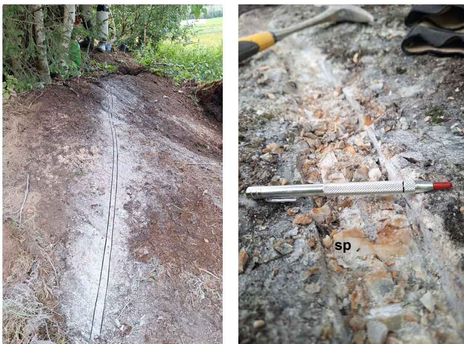
Figure 1: (left) Photograph of diamond cut channel at Orrvik facing south-southeast across strike; and (right) close up of one channel sample interval showing visible spodumene (sp) from channel sample OCSJF06 assaying 2.4% \text{Li}_2\text{O}
