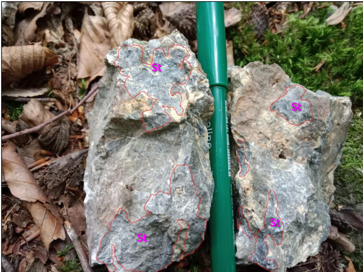
Figure 3. Antimony mineralisation at Krevia prospect with assays of 1.2% Sb (DM-014022) and medium-coarse grained stibnite minerals in hand sample (St). Mineralisation is hosted in breccia limestone replacing the host rock.
