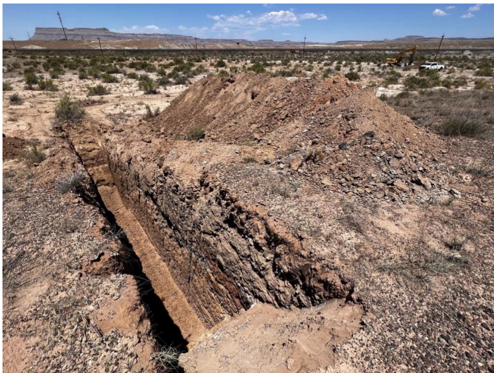
Figure 1: A photo showing one of the trenches completed for logging and sampling showing shallow bedrock.
