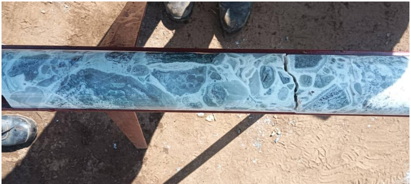
Figure 2: Breccia occurring at 188m(downhole) at Drill hole MPODD004. Sampling and assaying of MPODD004 (Anomaly Target 1) ongoing at the time of reporting.
