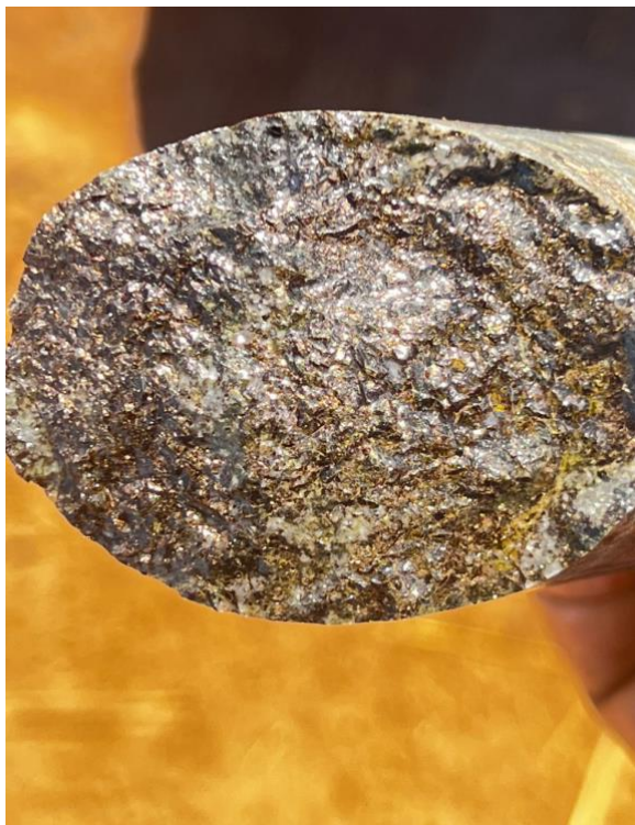
Figure 3: MPYDD001: Pervasive sulphide alteration/ mineralisation in NQ core at a depth of 85m downhole. Drilling and sampling of MPYDD001 (Anomaly Target 2) ongoing at the time of reporting.
