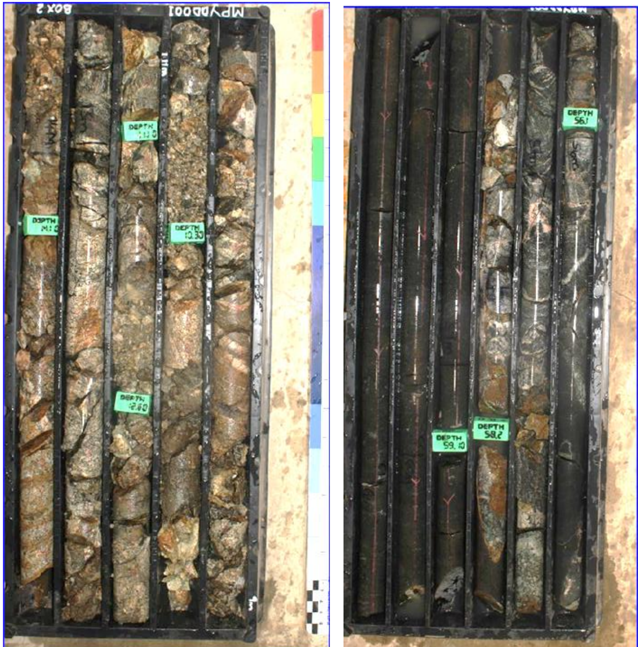
Figure 9 ; Mpyupyu anolmaly drillhole MPYDD001- (Left) Potassic alteration (fenitisation) and brecciation of wall rock adjacent intrusive system (9.3 to 14.3m downhole), Right - Barite rich dyke or stringer at 57 to 58 m down hole indicating increased sulphidation in the area. Drilling and sampling of MPYDD001 (Anomaly Target 2) ongoing at the time of reporting.
