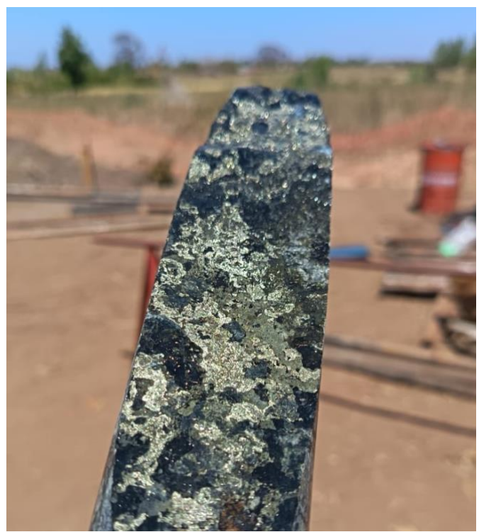
Figure 3: MPYDD001: Pervasive sulphide alteration/ mineralisation in NQ core at a depth of 85m downhole. Drilling and sampling of MPYDD001 (Anomaly Target 2) ongoing at the time of reporting.
