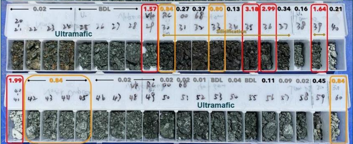
Chip samples from VKRC0068 and analysis results reported as g/t gold. 17m at 1.1g/t Au from 28m with higher grade intercepts up to 3.2g/t as annotated.
