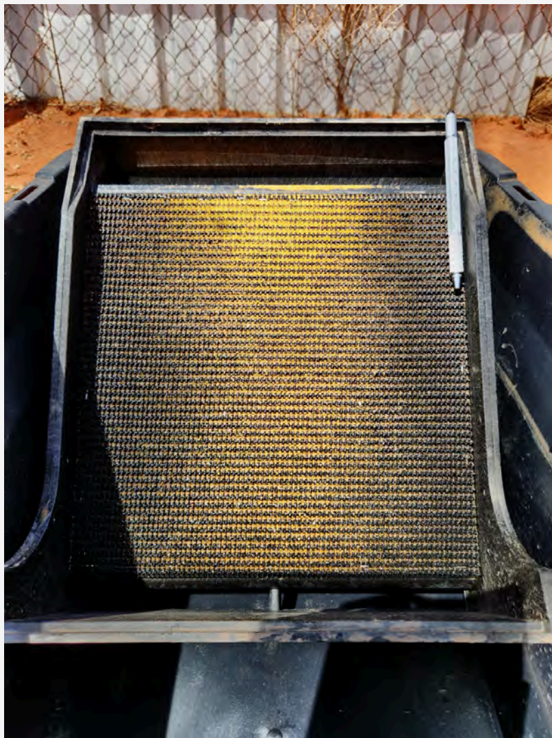
Picture 3. Pictures showing recovered gold at micro sluice*.
