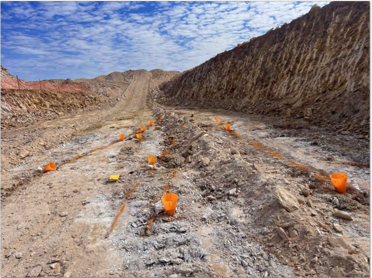
Picture 5. The orientation of mineralised quartz veins are indicated by orange lines drawn over the bulk sampling pit floor.
