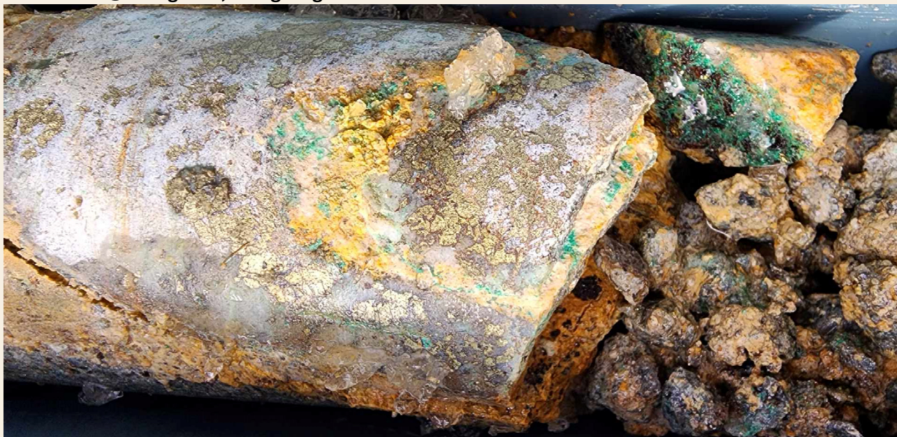
Figure 1. MRDD003 at 23.9m quartz vein with visible malachite and chalcopryrite, and goethite after sulphides, returning 0.5m @ 0.24g/t Au , 40.8g/t Ag & 3.7% Cu in assay.
