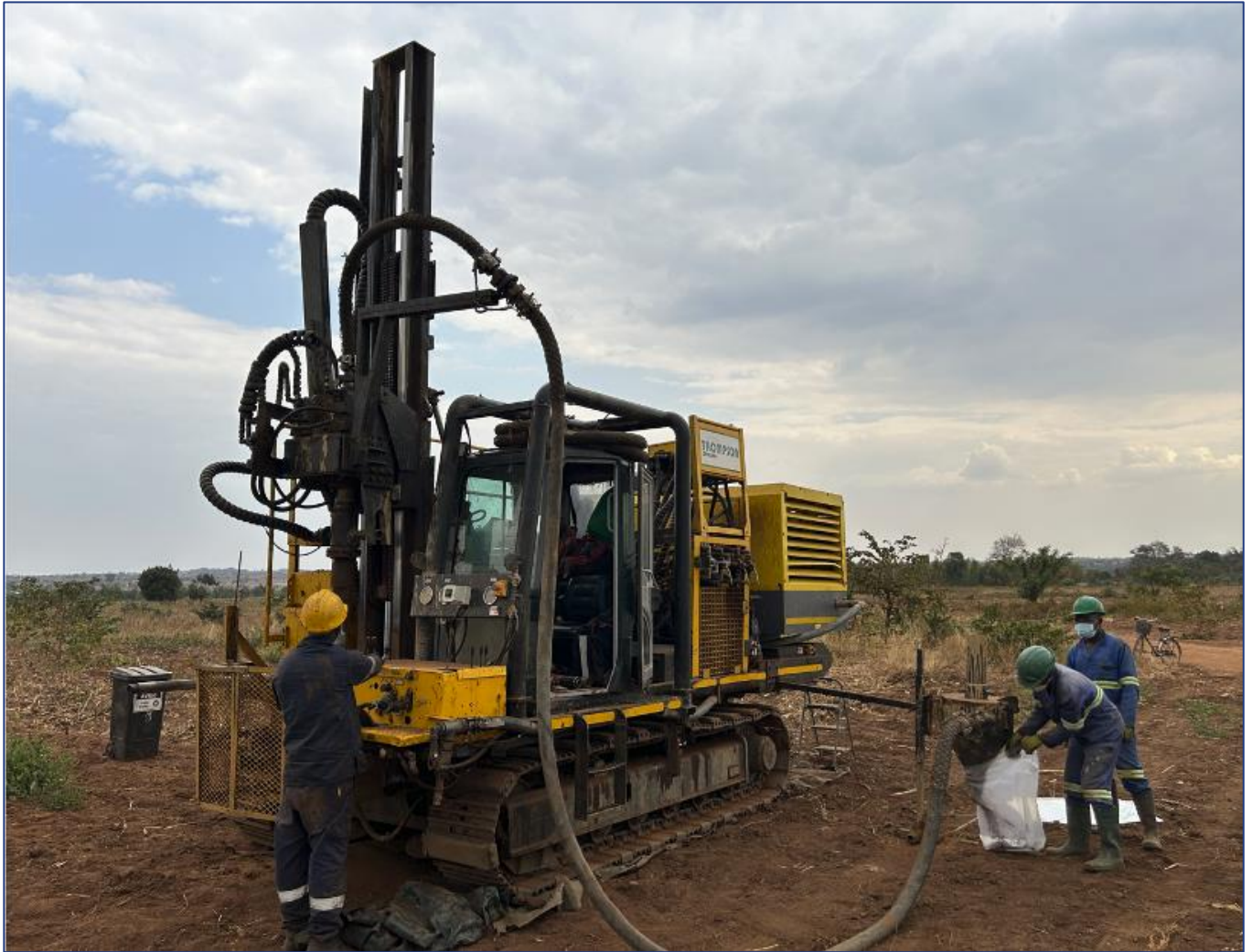
Figure 4: Commencement of a new hole using aircore drilling
