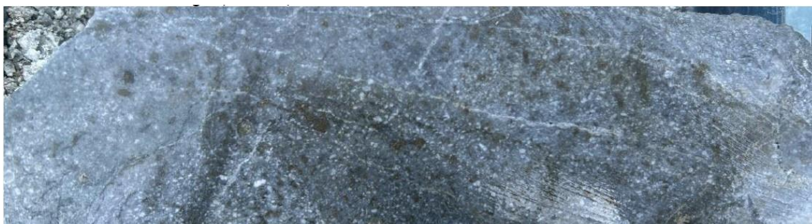
Figure 4 BISM0002 at 118.9m. Quartz-sericite-pyrite altered quartz monzodiorite. Visually estimated grade of the corresponding sample interval is approximately 0.1% Cu.
