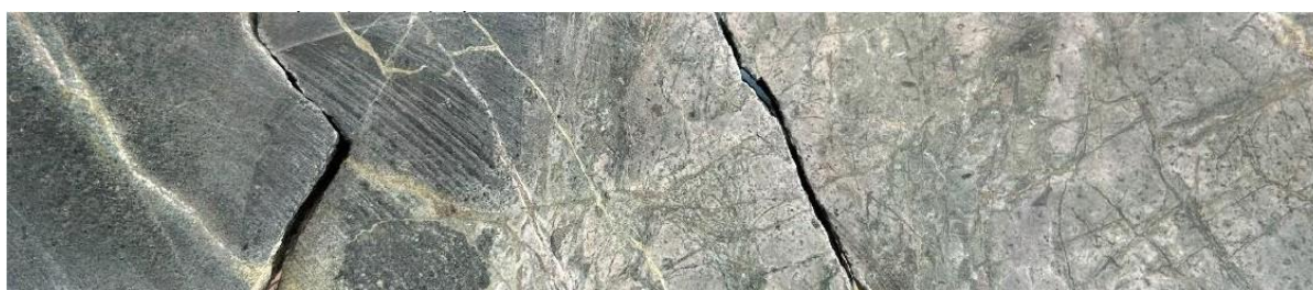
Figure 14 BISM0006 at 99.2m. Hornfelsed fine grained andesite with later epidote-chlorite and quartz-carbonate-pyrite veins. Visually estimated grade of the corresponding sample interval is approximately 0.1%Cu.
