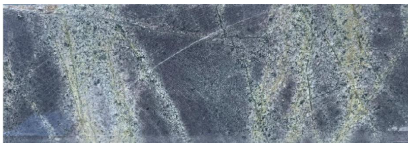
Figure 7 BISM0003 at 173m. Diorite with early potassic (biotite±k-feldspar) and later epidote-albite. Visually estimated grade of the corresponding sample interval is approximately 0.1% Cu.
