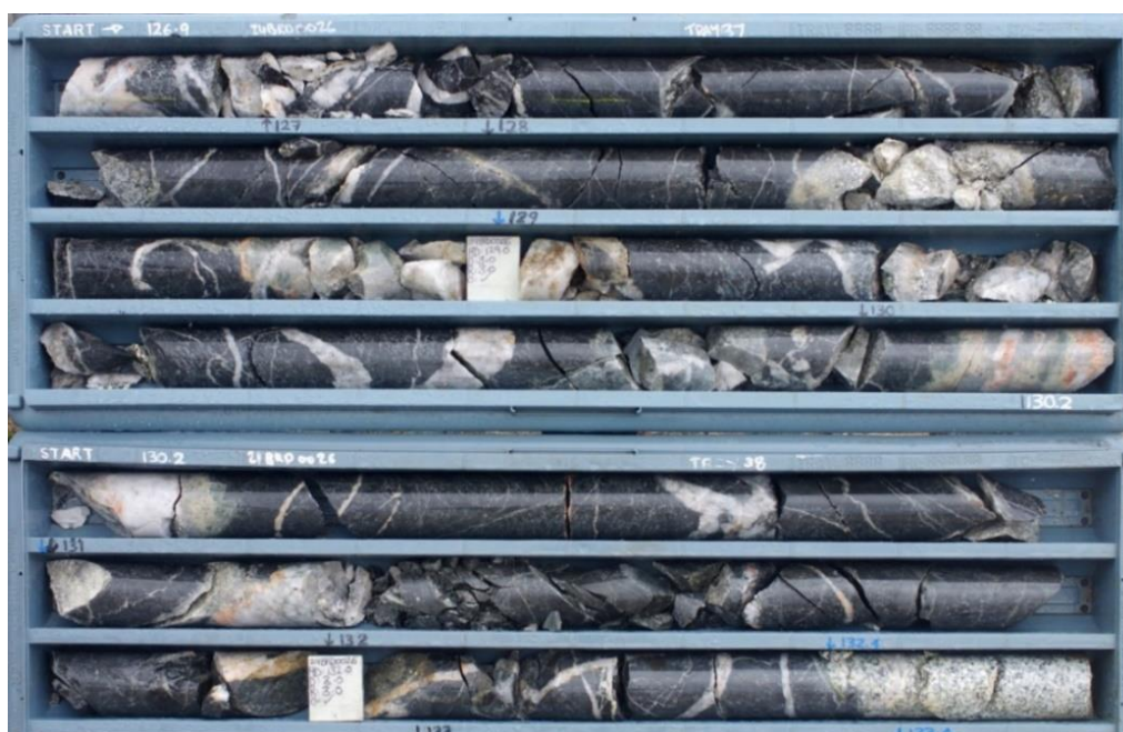
Figure 5 Mineralised volcaniclastic sediments immediately below the granodiorite contact. Note minor dykes of granodiorite and strong quartz veining. 24BRD0026 from 126.9m to 133.4m, weighted average grade 0.46% Cu.
