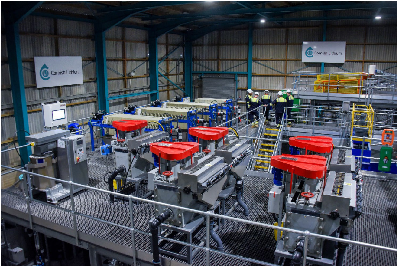
Figure 1: concentrator and filtration circuits, courtesy of Cornish Lithium
