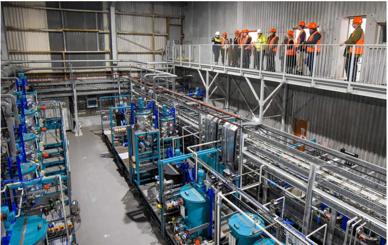
Figure 2: L-Max ® leach and impurity removal circuits, courtesy of Cornish Lithium
