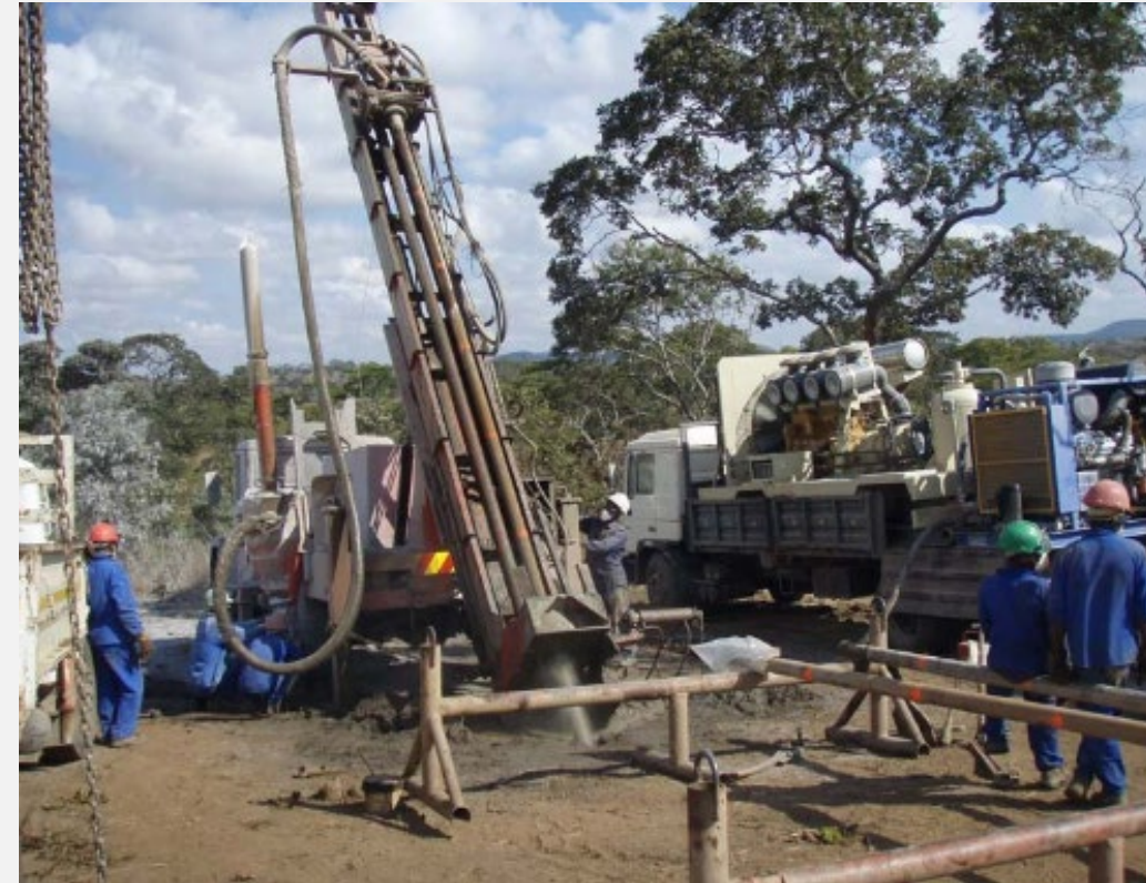
Exploration drilling on the Kanyika resource
