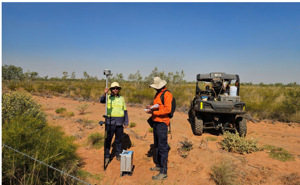
Figure 1. Atlas geophysics undertaking ground gravity surveying at the Christmas Creek Project.
