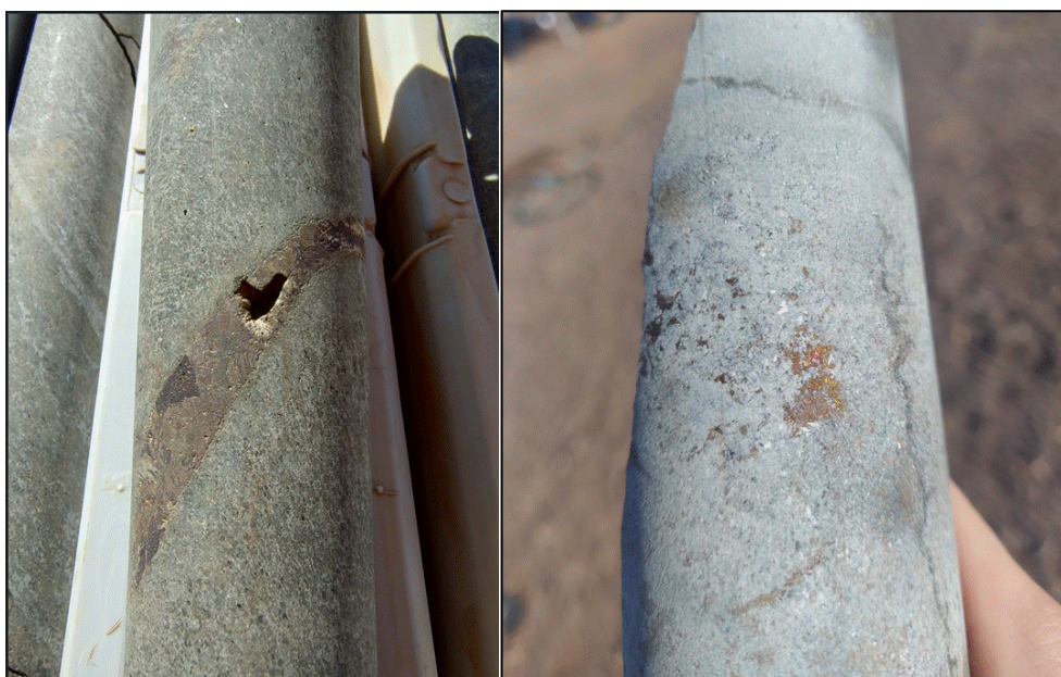
Figure 3a and 3b: Chalcopyrite and Pentlandite seen in cross-cutting veins in BUDD149 (left). Disseminated Bornite and Sphalerite in BUDD100 (right).
