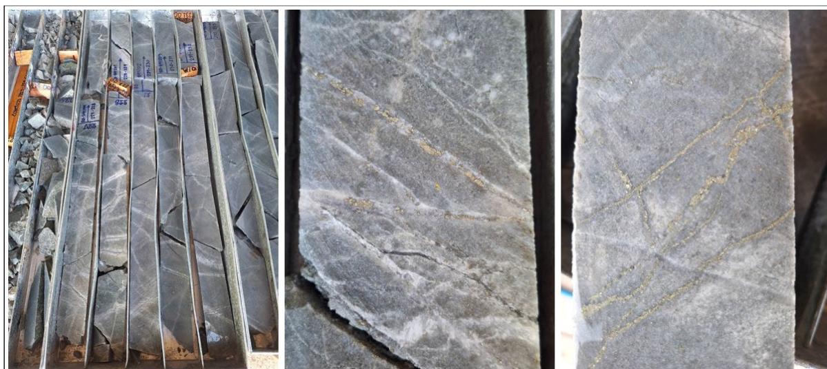
Figure 11: Quartz-pyrite stockwork veining towards the end of drillhole 7962RD.
