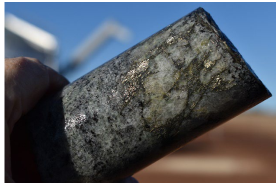
Photo 2: LRDD007 – 168m. Network textured pyrite associated with leucosome band within intermediate gneiss
