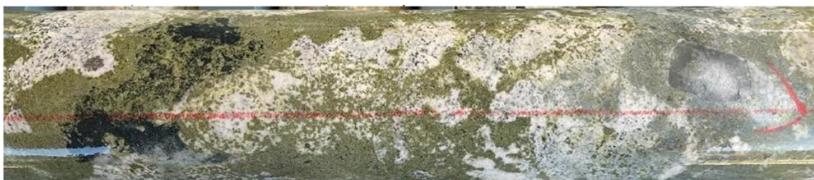
Figure 12 BISM0005 at 133m feldspar (albite?) -epidote-pyroxene (black) skarn alteration (refer Table 2).
