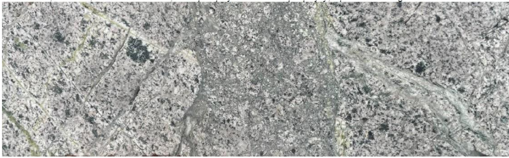
Figure 10 BISM0004 at 166m. Monzodiorite intrusive breccia dyke. Potassic (k-feldspar) alteration (refer Table 2).
