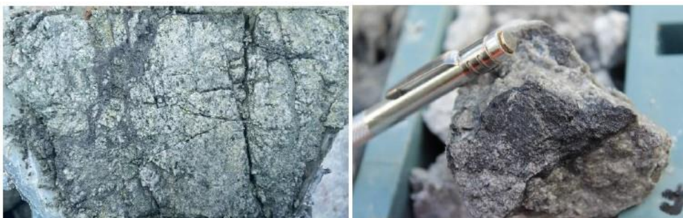
Figure 6 BISM0003 at 150m with grey molybdenite as fracture infill (refer Table 2).
