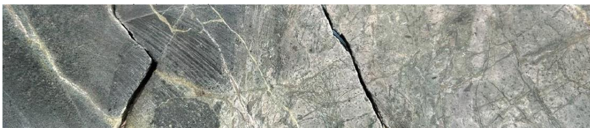
Figure 14 BISM0006 at 99.2m. Hornfelsed fine grained andesite with later epidote-chlorite and quartz-carbonate-pyrite veins (refer Table 2).
