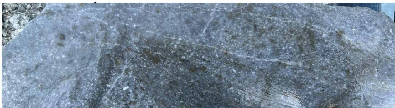
Figure 4 BISM0002 at 118.9m. Quartz-sericite-pyrite altered quartz monzodiorite (refer Table 2).
