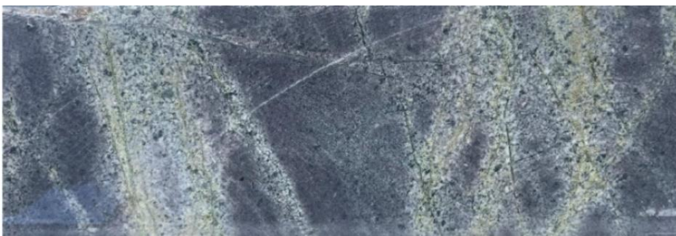
Figure 7 BISM0003 at 173m. Diorite with early potassic (biotite±k-feldspar) and later epidote-albite (refer Table 2).
