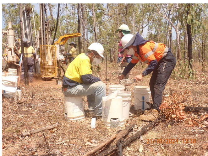
Figure 2: Reverse Circulation Aircore drilling underway at Alice River Gold Project
