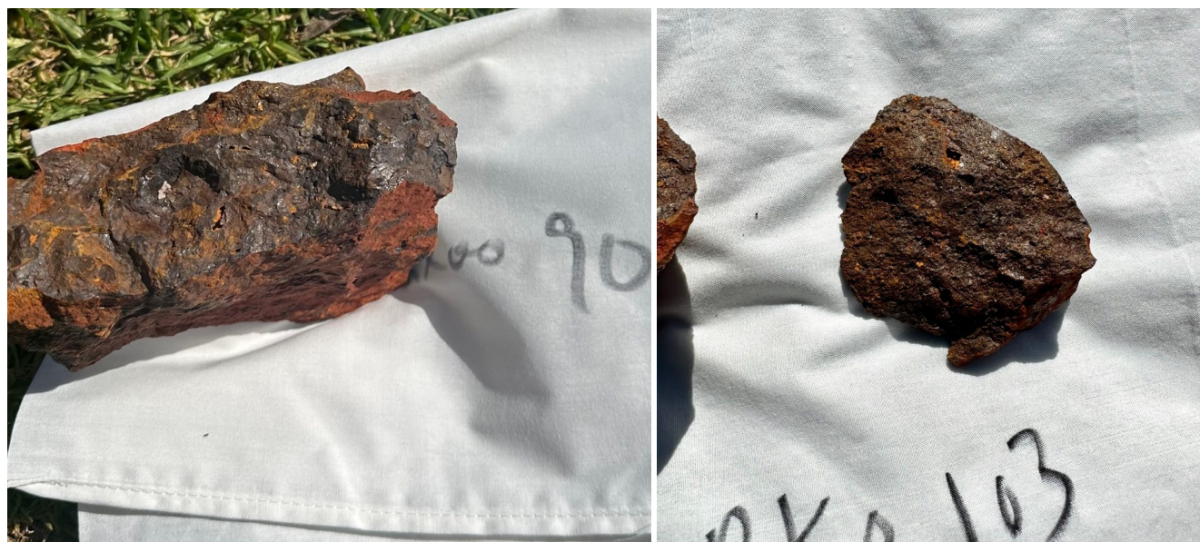
Figure 4: PWRK0090 (left) returned 55.27% Fe, PWRK0103 (right) returned 53.73% Fe
