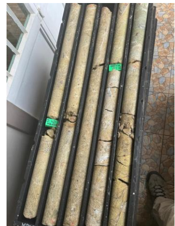
Figure 3 Diamond core. Lithology is predominantly nepheline syenite with a pervasive carbonate veining from around 75m to end of hole at 122m (see Appendix 4).
