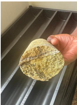
Figure 1 Diamond core, weathered nepheline syenite at 87m with carbonate veining. See further commentary in Appendix 4.
